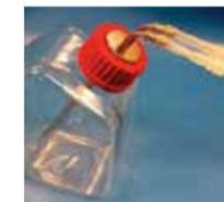
**45 mm (Cat # A1008) -** Reservoir Cap Assembly fits Gibco® media bottles. The assembly includes a 516 stainless steel cap assembly with two angled tubes, a 45 mm threaded sealing ring and one white silicone gasket to seal the bottle firmly against the cap for leak proof operation.
