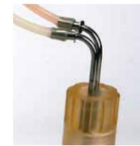
**38 mm (Cat # A1006) -** Reservoir Cap Assembly fits standard plastic media bottles. The assembly includes one medical grade polysulfone cap with molded-in silicone plug, two 516 stainless steel delivery tubes and one .062" thick white silicone gasket. Withstands repeated autoclaving.
